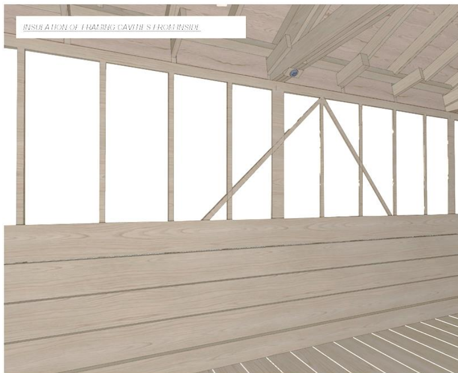
Figure 8 - Architect’s rendering illustrating how Options 3 and 4 would look e.g. board insulation installed inside between the wood studs with new metal panels glued to the front face of insulation to replicate the look of the back side of the metal siding. Although some wall depth between the wood studs is lost, the pattern of the wood studs and rail boards are still visible.
