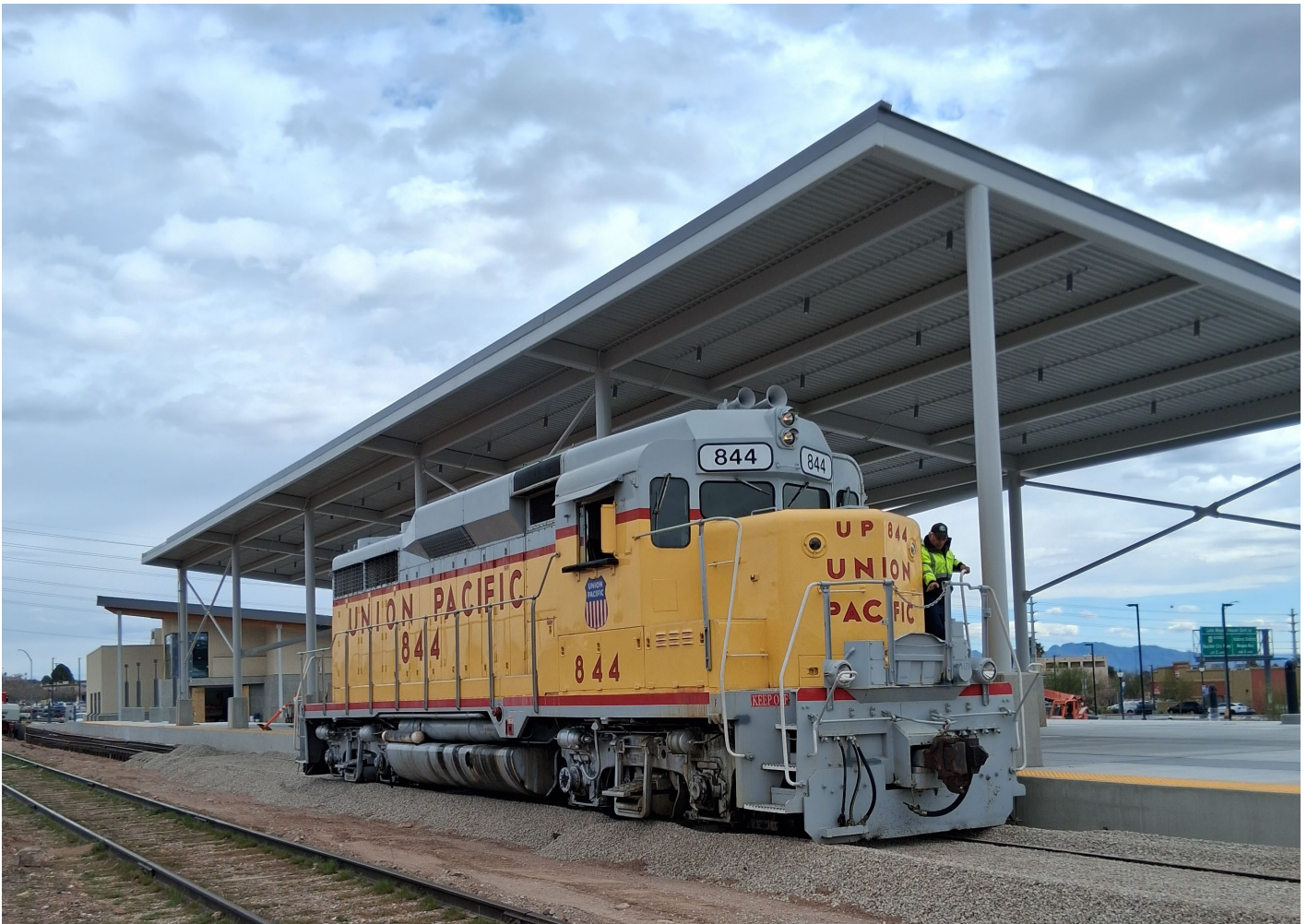
Locomotive 844 tests clearances on the new siding for the visitor center passenger platform.
